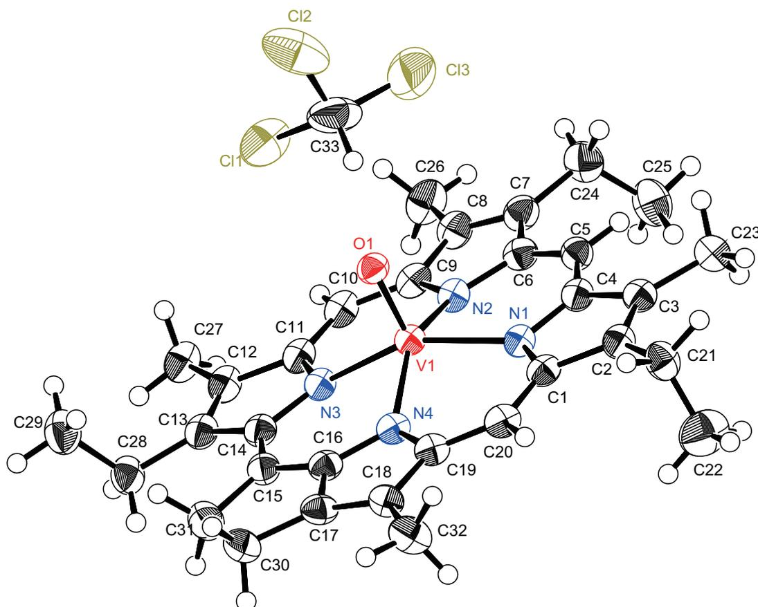
Fig. 5. X-ray crystal structure of vanadyl DPEP. Dark red block crystals of  $C_{30}H_{30}N_4OV$  were grown by vapor diffusion (methanol into  $CHCl_3$  solution). A single crystal with the approximate dimensions of  $0.15 \times 0.12 \times 0.07$  mm was then mounted on a glass fiber. Measurements were made on a Rigaku RAXIS RAPID imaging plate area detector using graphite monochromated  $Cu K\alpha$  radiation.
