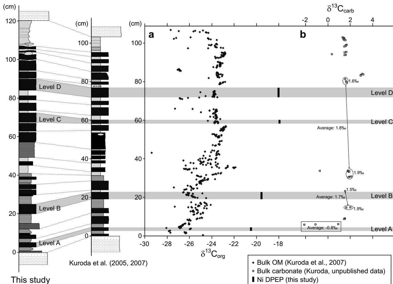
Fig. 6. Stratigraphic column of the Livello Bonarelli black shale at the Gorgo Cerbara section based on data from the present study and Kuroda et al. (2005), showing Kuroda et al. (2005)  $\delta^{13}\text{C}$  data for (a) bulk organic matter and (b) bulk carbonate. (For interpretation of the references to colour in this figure legend, the reader is referred to the web version of this article.)
